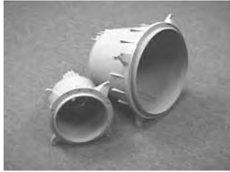
**Gunite Plastic Niches** - These plastic concrete niches are molded of high strength, corrosion resistant PVC with a one inch PVC hub. Both 45O and 3/4 in. reducer bushings are included. Gunite models feature rebar tie-backs and a plaster ring for clean, simple installations and all are packed with a gunite/plaster shield.
